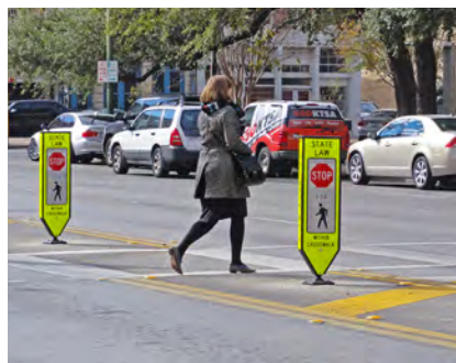
In-Street Pedestrian Crossing Signs
