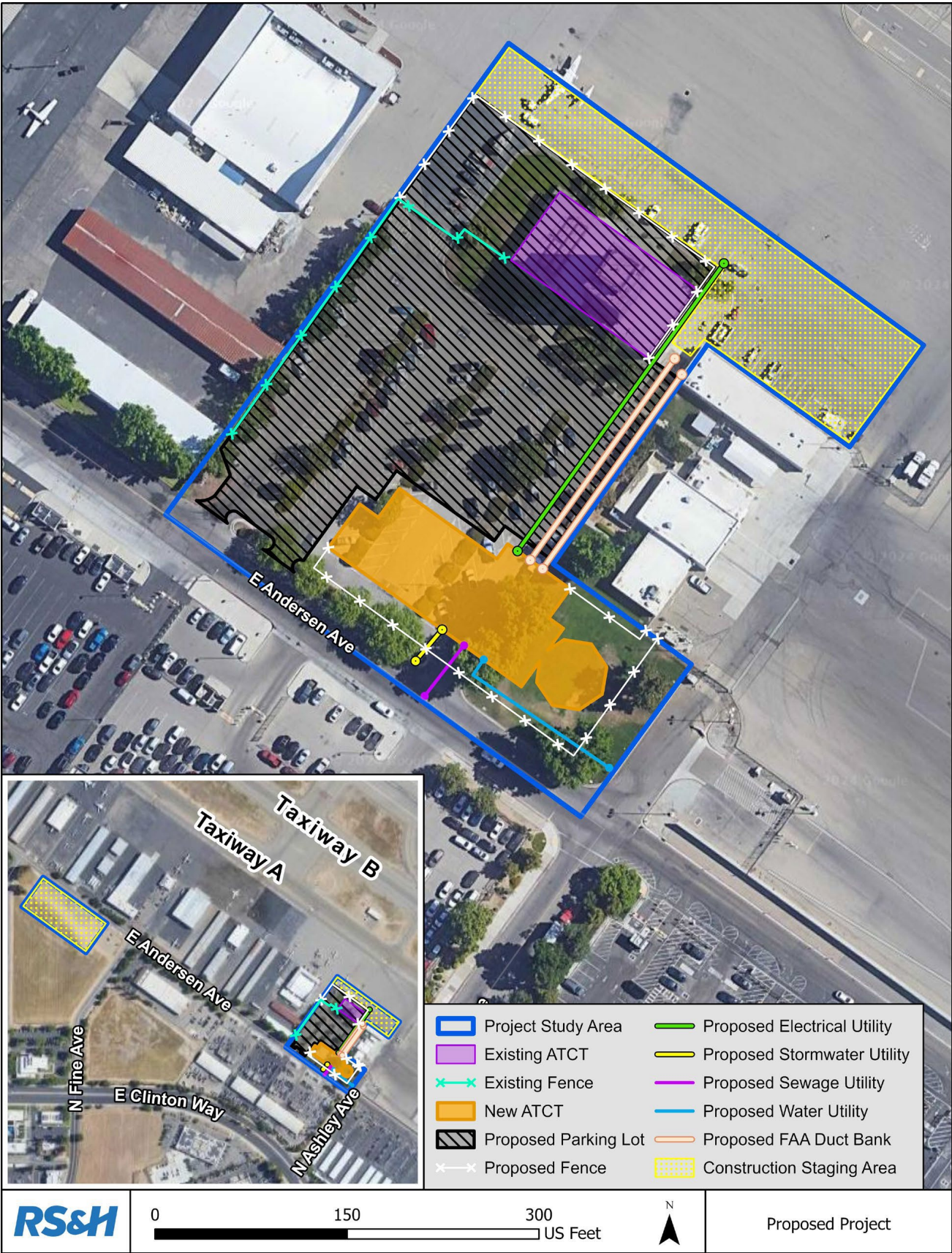
Exhibit 1: Proposed New Airport Traffic Control Tower
