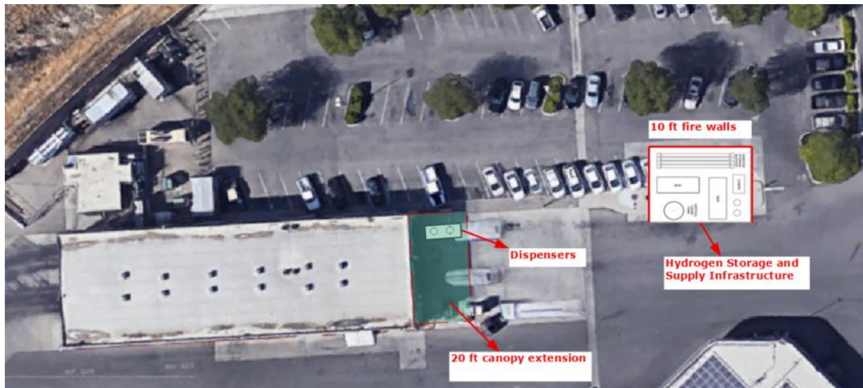
Figure 5: Satellite overhead view of hydrogen infrastructure placement
