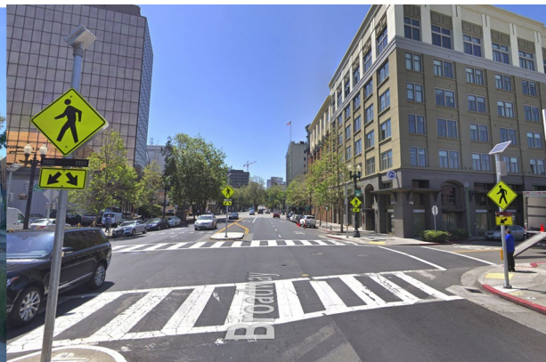
Figure 3.10: A Pedestrian Rectangular Rapidly Flashing Beacons (RRFBs) in Oakland CA (Source: Google Streetview)
