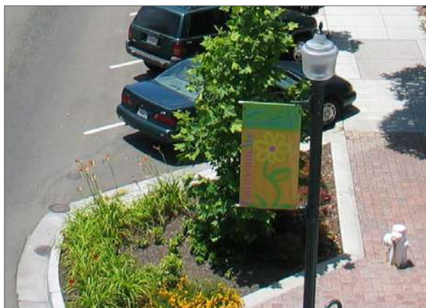
Street tree bulbout in an angled parking lane.
