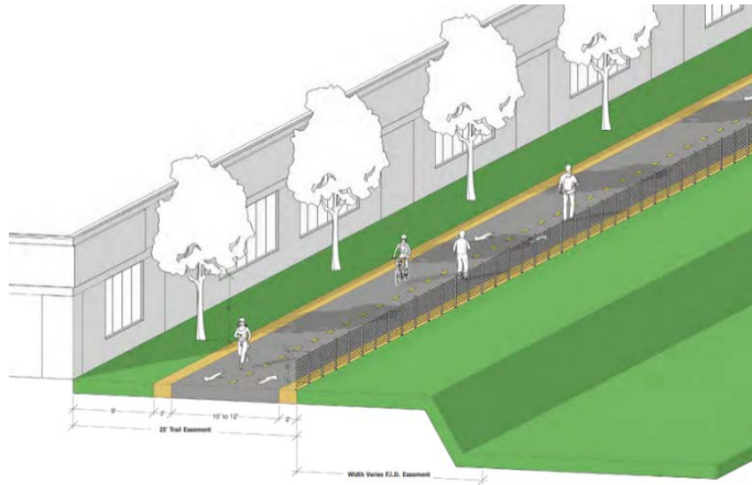
Figure 16. City standard canal side trail section
