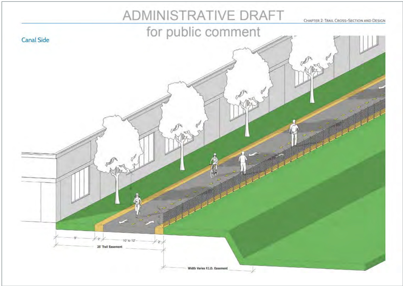
Figure 7. Typical Cross Section for Class I Canal Side Trail: City of Fresno Trail Design Guidelines
