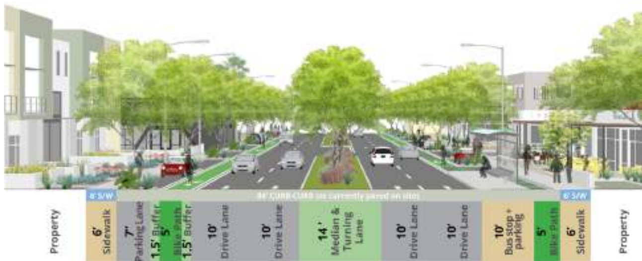
Figure 4-7. Existing and Proposed Street Design for Kings Canyon Road
