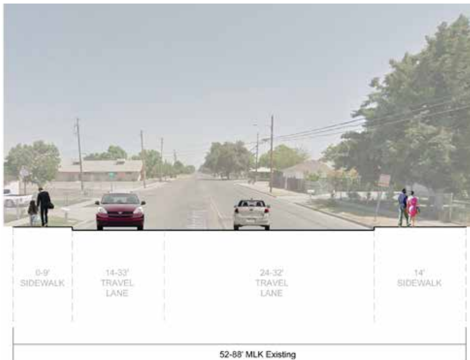
Figure 2.9: Existing Martin Luther King Blvd Cross-Section
