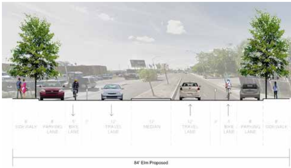
Figure 3.23: Elm Avenue Cross-Section
