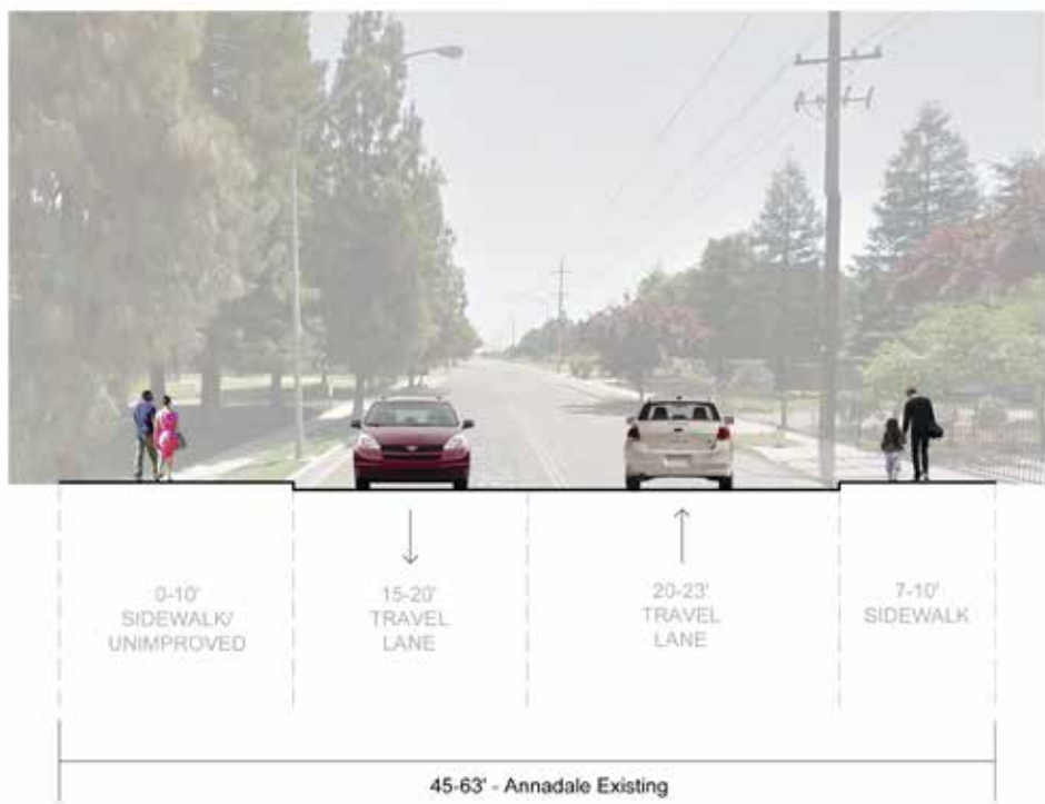
Figure 2.8: Existing Annadale Avenue Cross-Section
