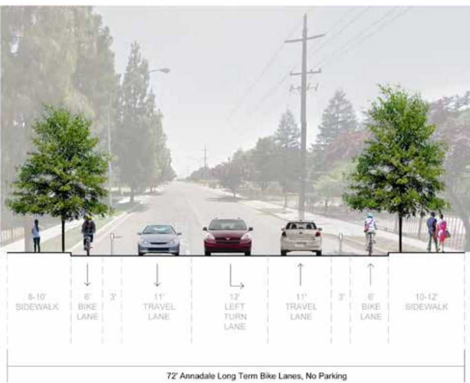
Figure 3.18: Annadale Avenue Long Term Cross-Section
