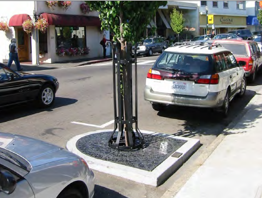
Planting street trees within bulb-outs are ideal when sidewalks are too narrow to accommodate them, in addition to being a great tool for reducing automobile traffic speed.
