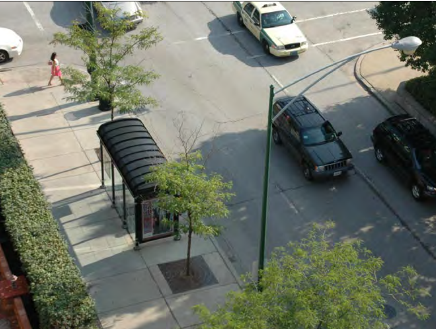
A bus shelter constructed of quality materials. Glass floor to ceiling panels improve the perceived safety of waiting passengers. Adjacent street trees provide additional shade.
