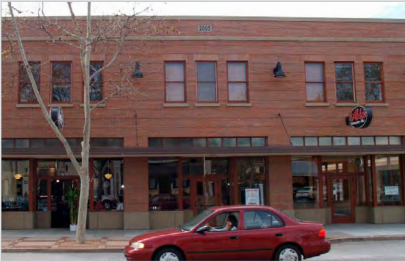
The windows of this mixed-use building are composed according to a logical order. The second floor windows are grouped in threes and centered above the ground floor shopfront doors and windows.
