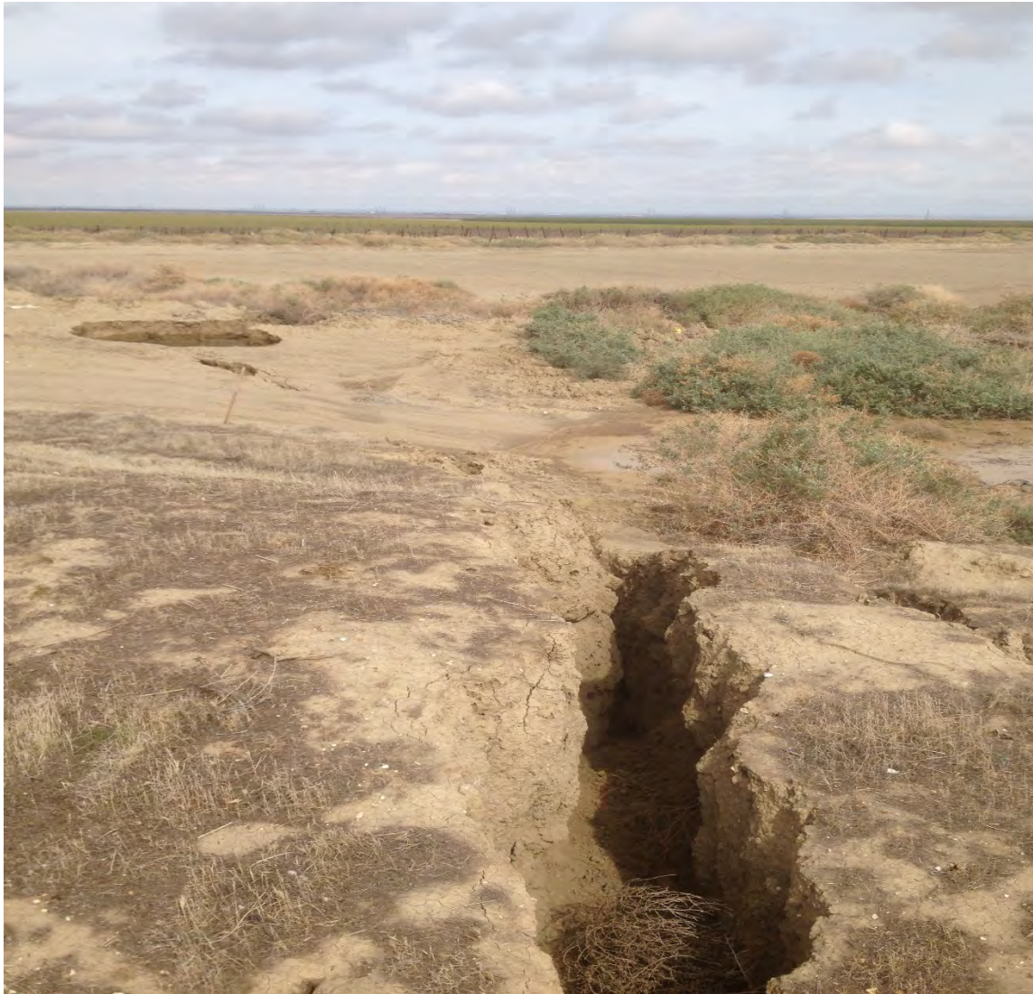
Figure Q.5: Lateral 7r-4.5 Subline Earth Movement Caused Fracture and Pipeline Blow
