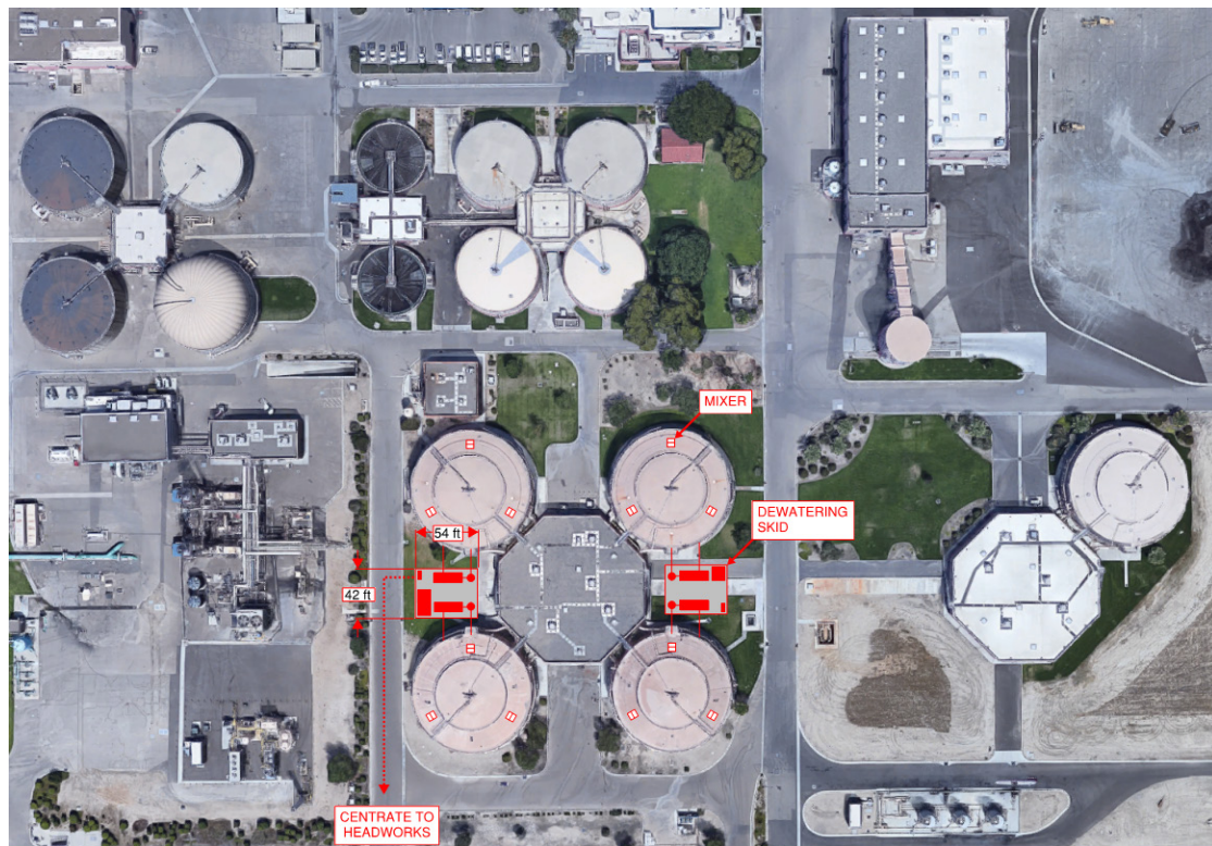
Figure 4.5 Baseline: MAD with Recuperative Thickening Site Layout
