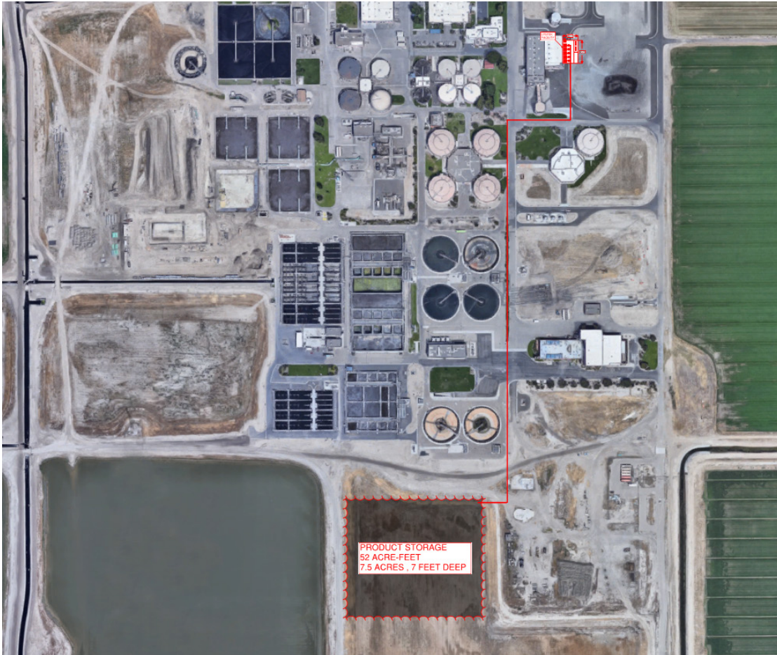
Figure 4 10 Post-Digestion Thermo-Chemical Hydrolysis – Onsite Site Layout
