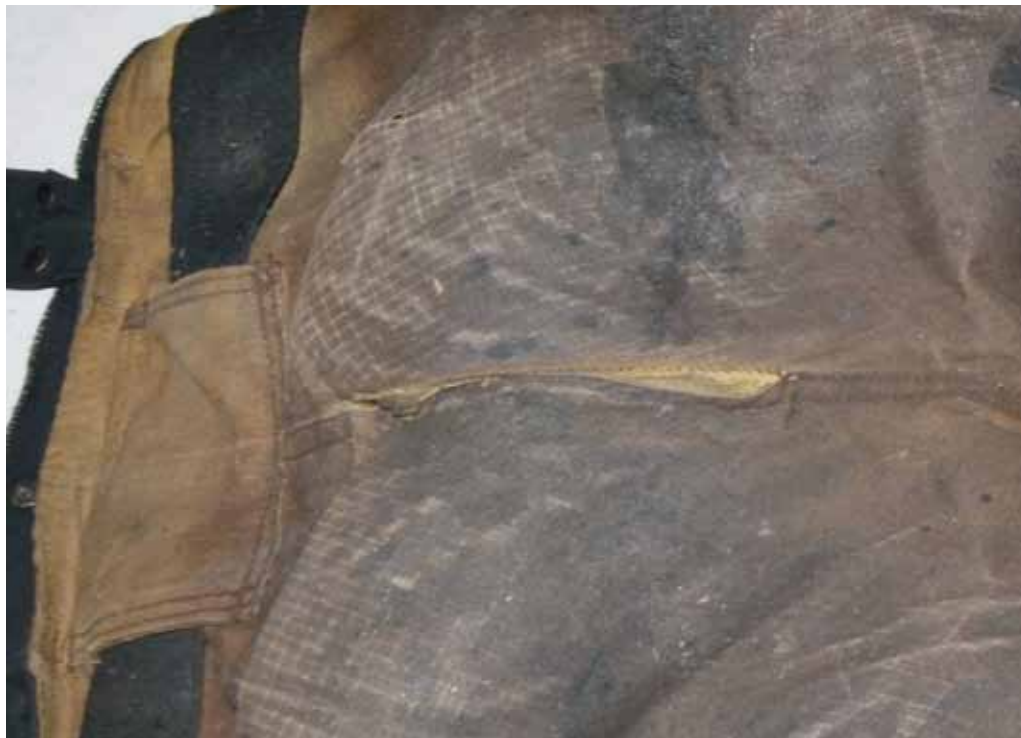
Figure 28: Seam failure in seat of pants
