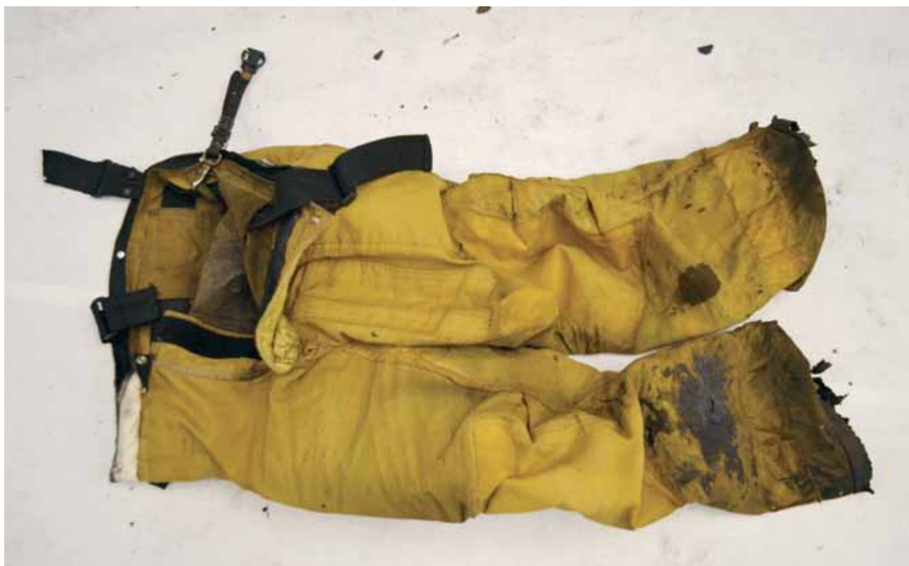
Figure 32: Outershell of pants turned inside-out showing thermal damage to lower leg and cuffs
