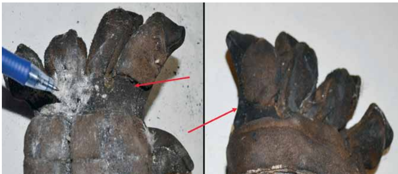
Figure 3: Visible indentations around the fingers of both gloves
