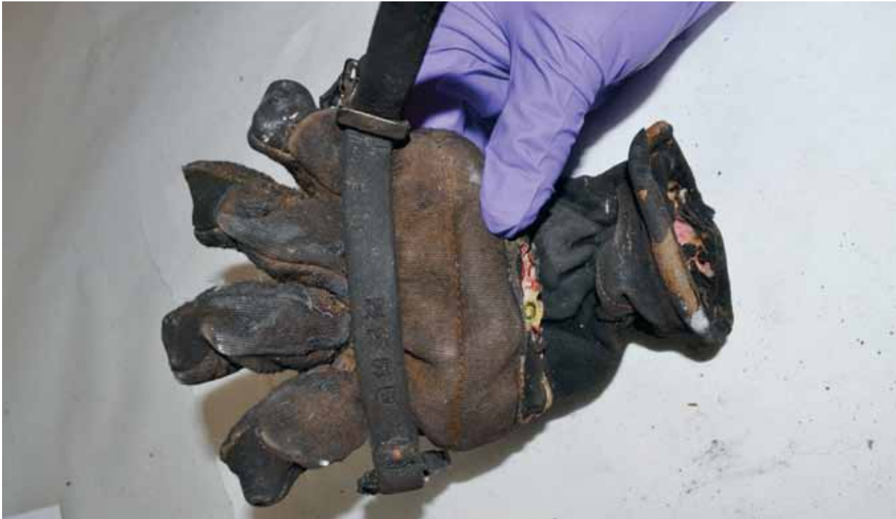
Figure 5: Leather glove strap aligns with indentations on glove (top view)
