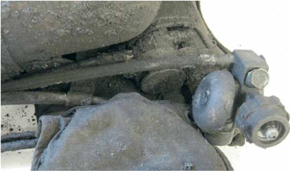
Figure 13: High pressure line and cylinder attachment.
