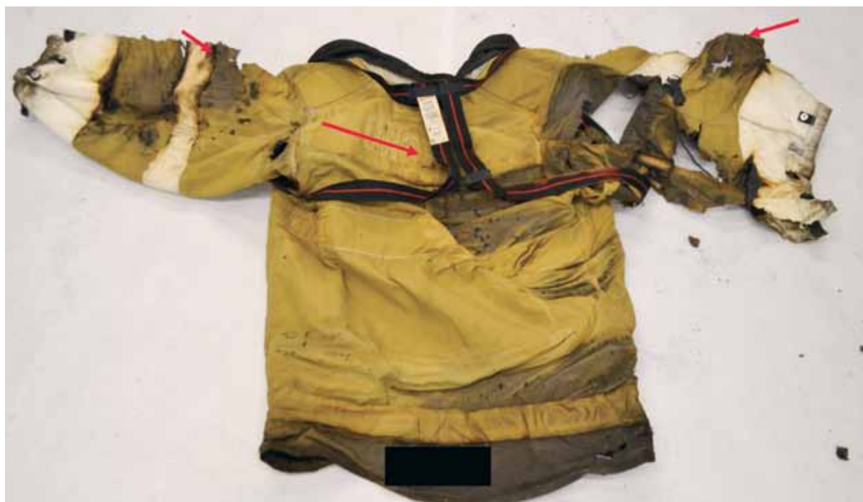
Figure 18: Coat shell turned inside-out showing the DRD installed properly and thermal break open on sleeves
