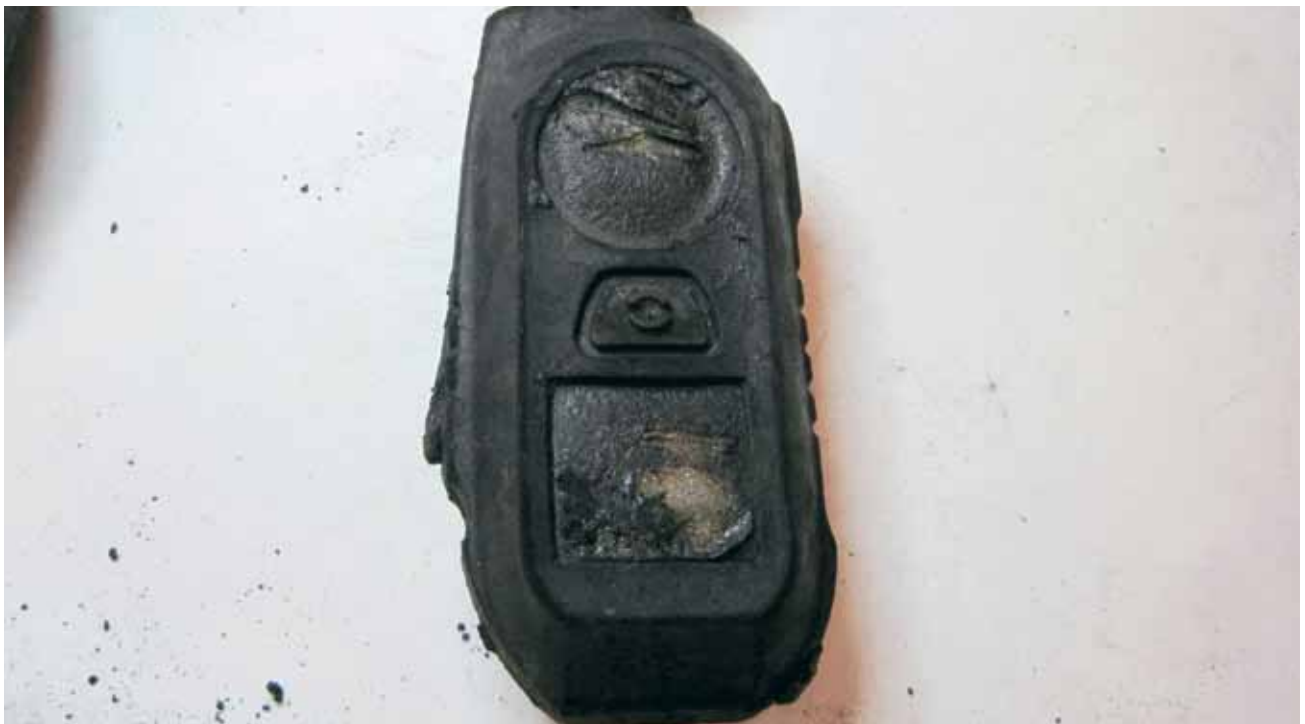
Figure 16: Significant heat damage to PASS console.
