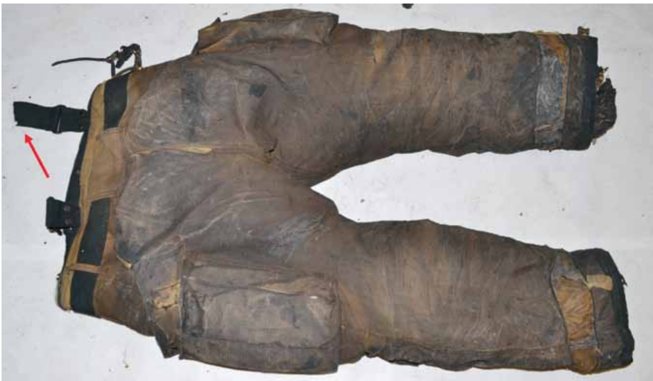
Figure 26: Suspenders were cut and substantial thermal damage visible to back of pants including reflective trim at cuffs
