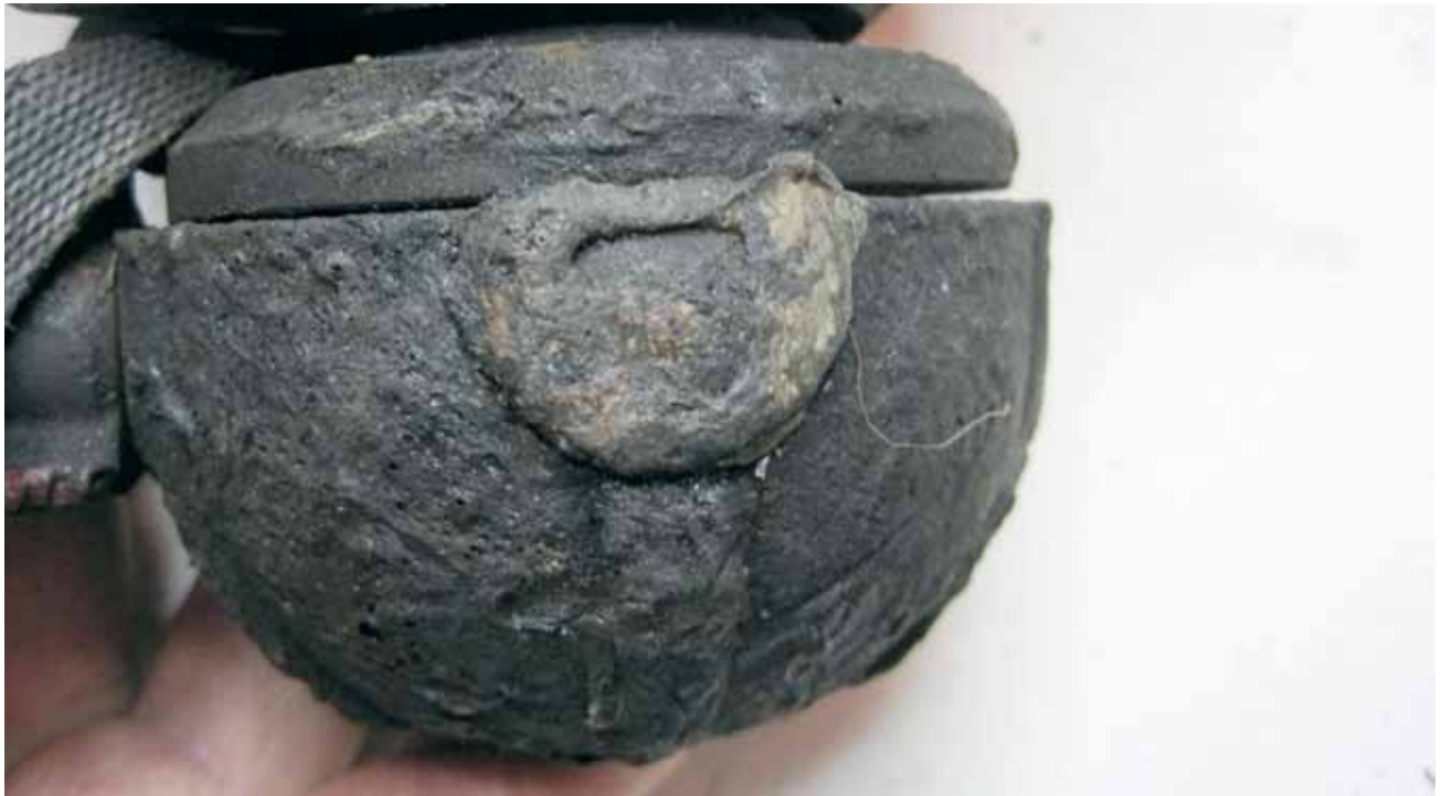
Figure 8: Melted top locking point.
