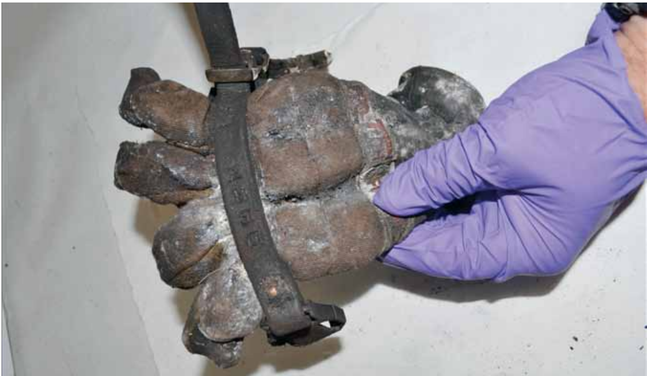
Figure 6: Leather glove strap aligns with indentations in glove (palm side)
