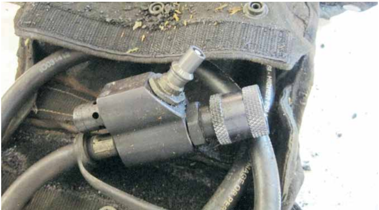
Figure 28: Both auxiliary hose fitting uncapped and clean.
