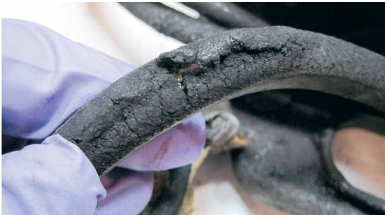
Figure 9: Low pressure hose possibly compromised.
