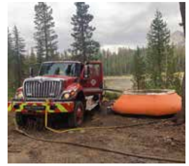
Type III brush engine drafting from a portable tank
