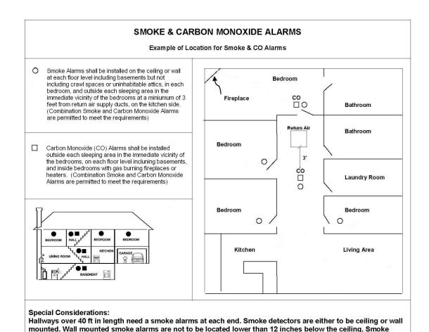
alarms are not to be mounted within 4 inches of a wall/ceiling corner.
