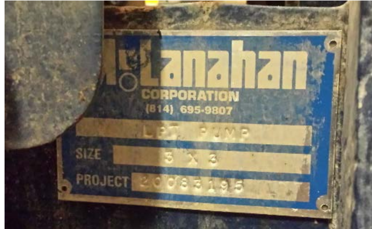
Figure 5.26: Solids Pump Nameplate
