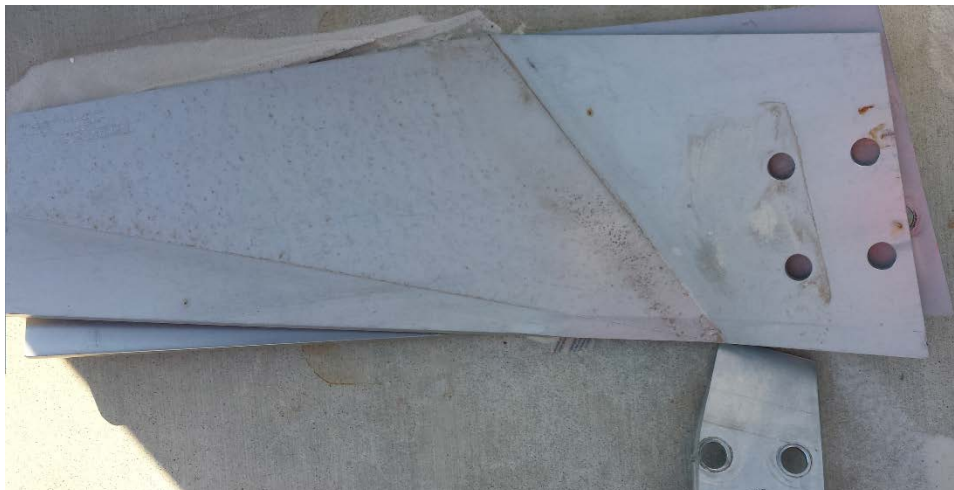
Figure 5.18: Example of the Injection Mixer Broken Blades
