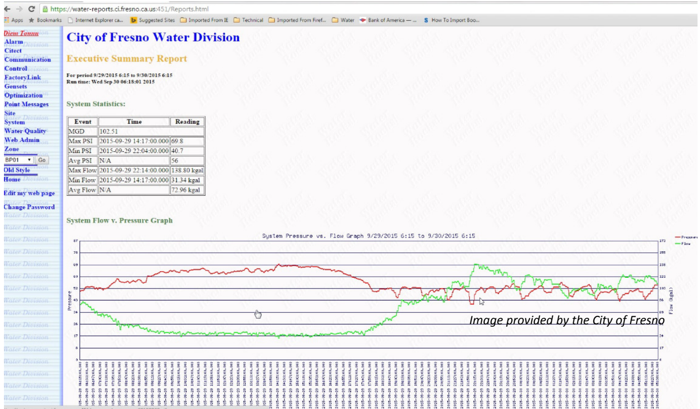
A SCADA graph showing system pressure (red) vs Flow (green) over a twenty-four hour period This is just one of many data views available through SCADA
