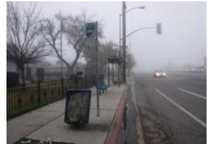
5. **Boarding and Alighting Dimensions:** The space between the curb edge and the back of the existing sidewalk was not at least 96” deep, where the additional space appears to exist in the adjacent property.
