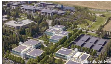
BUILDING-INTEGRATED PHOTOVOLTAICS. Rooftop or integrated solar panels can effectively supply energy to groups of buildings, as with the 1.6-megawatt array at the Google headquarters in Mountain View, which is capable of serving 30 percent of peak demand.
