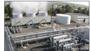
BIOGAS. Anaerobic digesters can produce biogas and/or electricity from animal waste or other organic matter.
