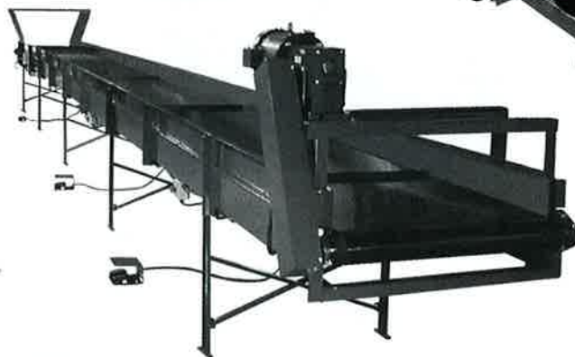
Custom 36 in. x 50 ft. sorting conveyor
